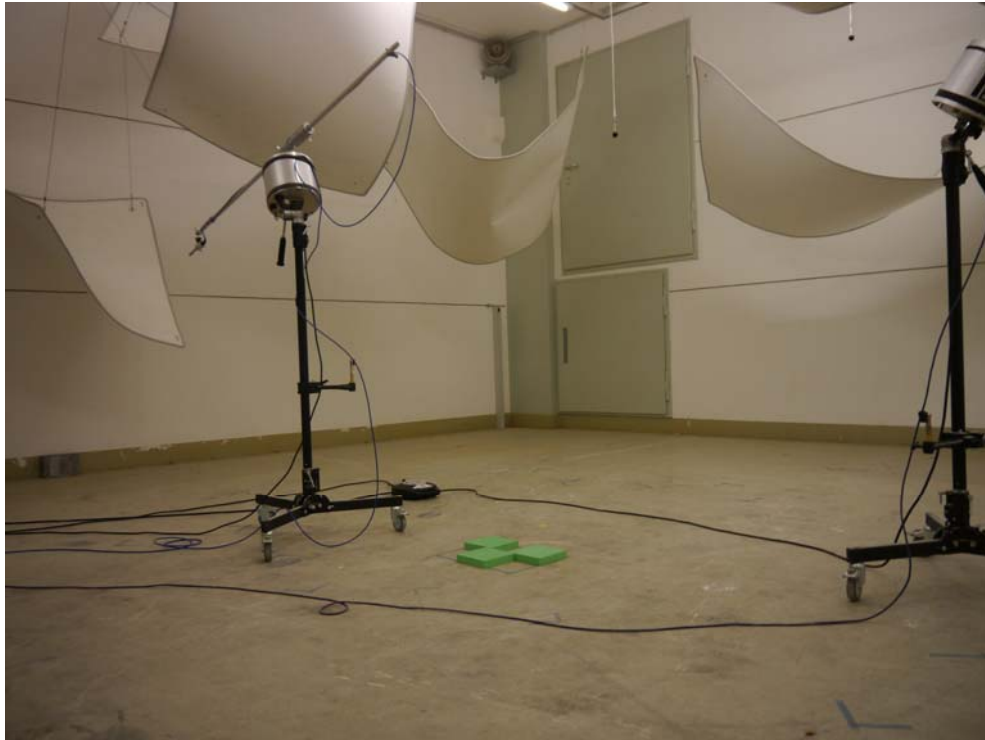
Figure B.1. Reverberation room and test position without test object.
