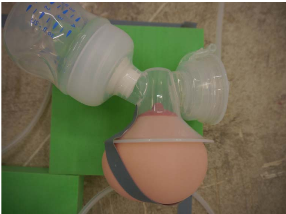
Figure B.4. Suction bottle with fixed artificial breast.
