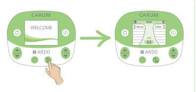
Express mode starts with an especially mild, gentle and low suction strength and suction frequency.
